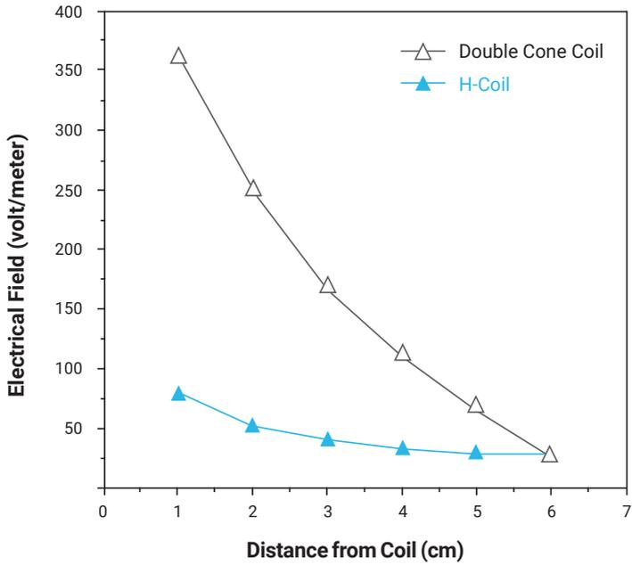
Induced electrical field plotted as a function of distance for the double-cone coil and the H-Coil. Although the double-cone coil produces a much larger induced field, the rate of decay of the field with distance is much smaller for the H-Coil. This allows the H-Coil to stimulate deeper brain areas without inducing an intolerable electric field in more superficial brain areas.
